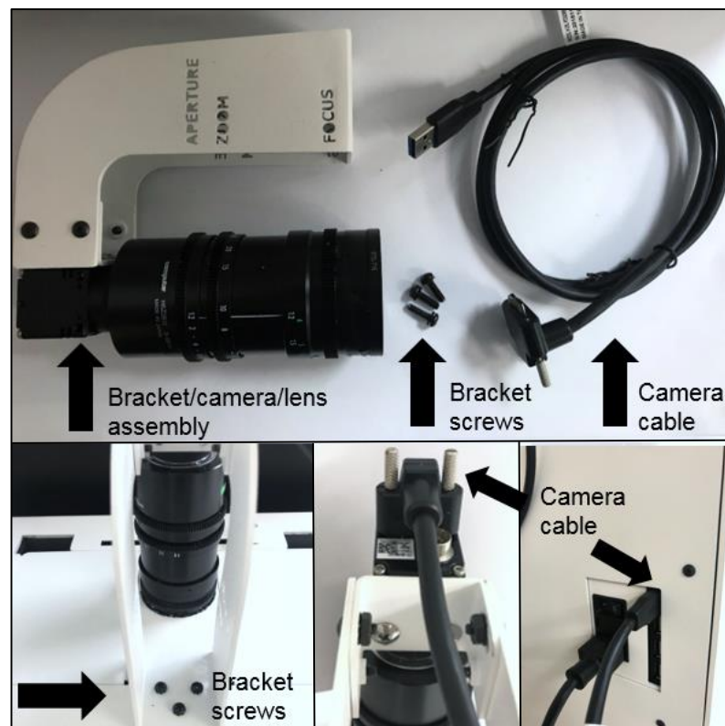
Fig. 6 Connecting the camera bracket/camera/lens assembly
